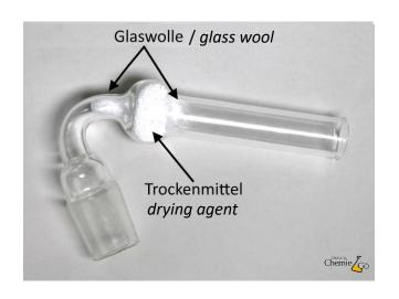
Subsequently, the sphere is filled with a drying agent (e.g. CaCl<sub>2</sub>) and closed up with glass wool.
