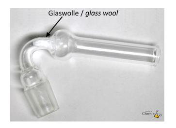
The sphere of the drying tube is plugged with some glass wool to prevent the drying agent from entering into the apparatus.
